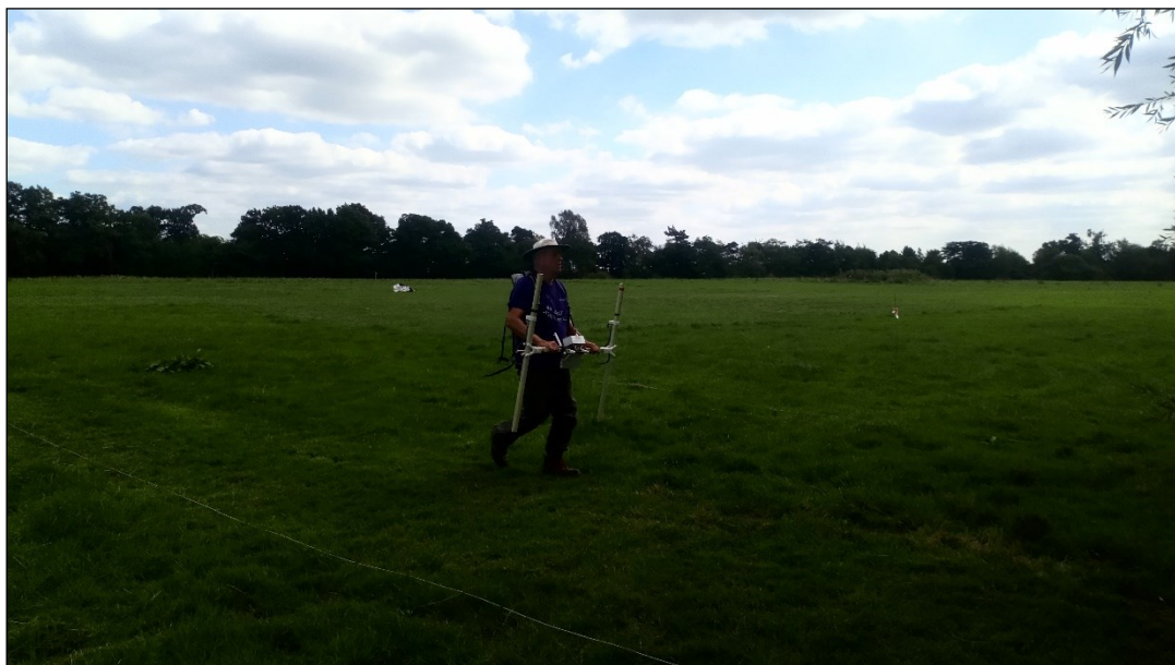
Figure 6 Magnetometer survey being conducted using a Bartington Instruments Grad 601 fluxgate gradiometer (photo: K. Strutt)
