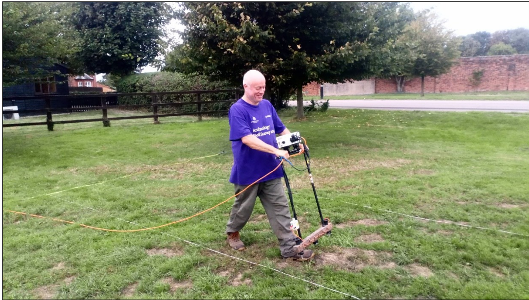
Figure 7 Earth resistance survey being carried out using a Geoscan Resesarch RM15 (photo: K. Strutt)
