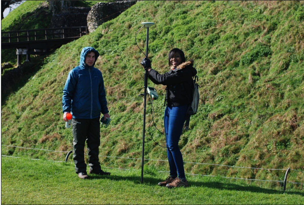
Figure 5 Leica RTK GPS with Smartnet being used to grid out (photo: K. Strutt)
