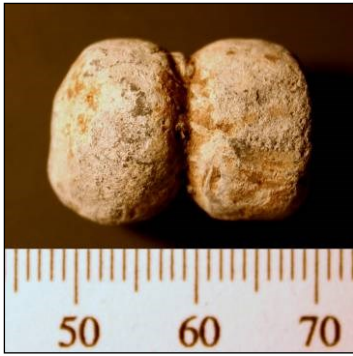
Figure 4: two probably originally spherical lead bullets apparently fused and compressed by being fired as a double load (find 8)
