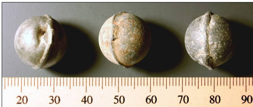
Figure 3: bullets with high intact flash ridge and very limited surface corrosion. Probably more recent bullets. The left bullet shows incomplete fill of mould adjacent to sprue snip.
