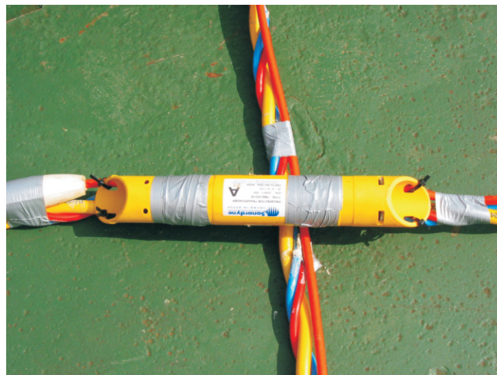
Plate 3: SCOUT beacon on umbilical
