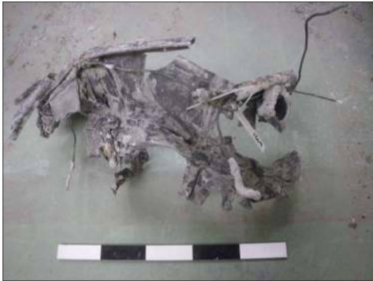
Plate 1: Damaged cockpit instrument console
