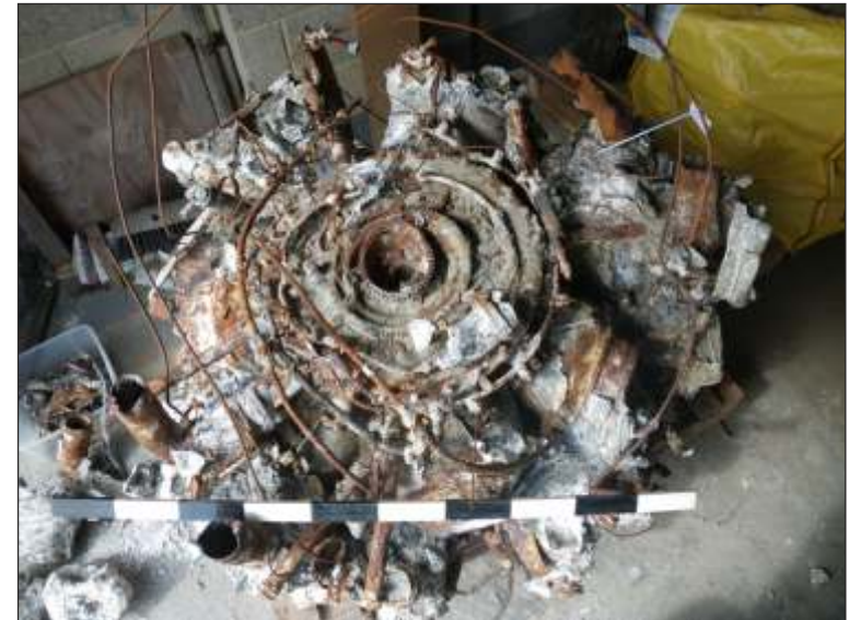
Plate 4: BMW 801 14 cylinder radial engine (probably a G-2 version)
