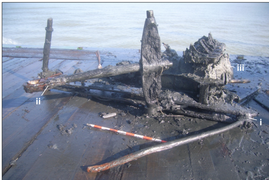
C: WA3048 side lever beam (i), WA3049 crosshead (ii) and WA3050 pump (iii)
