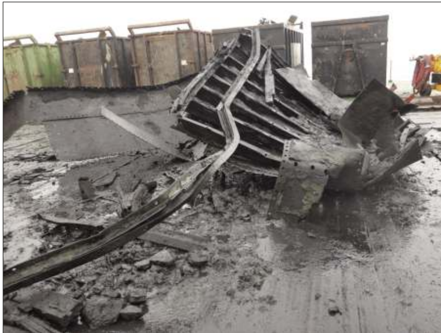
Plate 3: Section of hull with iron riveted plating, frames and stringers, WA3152
