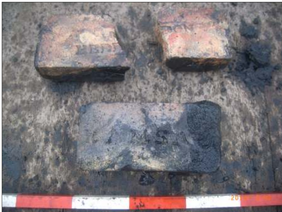
Plate 2: Firebricks with Tyne and Wear manufacturer's marks; 'Heddon' and 'Ramsay', WA3010
