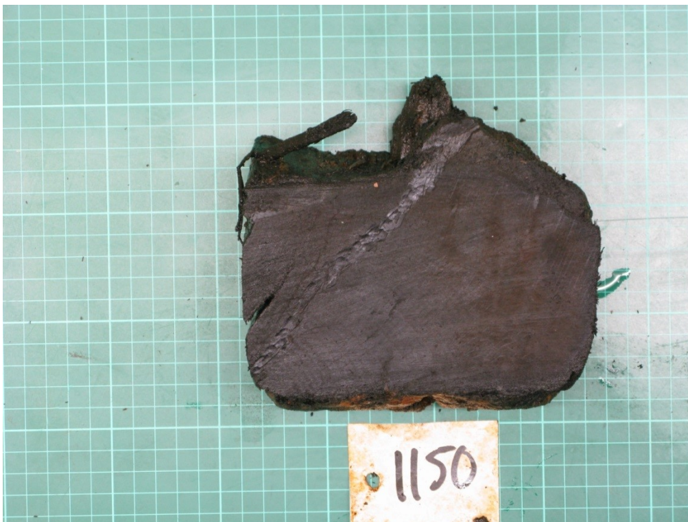
Figure 13 Photograph of LG1150 sample. Sapwood is visible in outer right top corner
