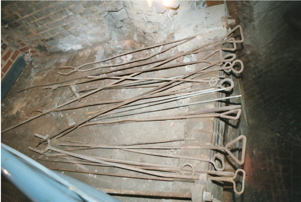
Figure 3.17: A selection of glassworkers' tools (Red House Cone)
