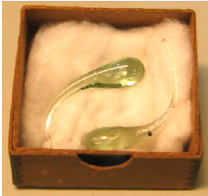
Figure 3.34: Prince Rupert's drops (approx 2 x actual size)
