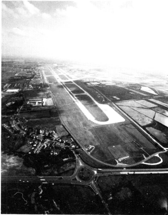
Plate 1. Aerial view of Heathrow Airport, looking east. The aircraft holding area and runway extension are nearest to the camera.
