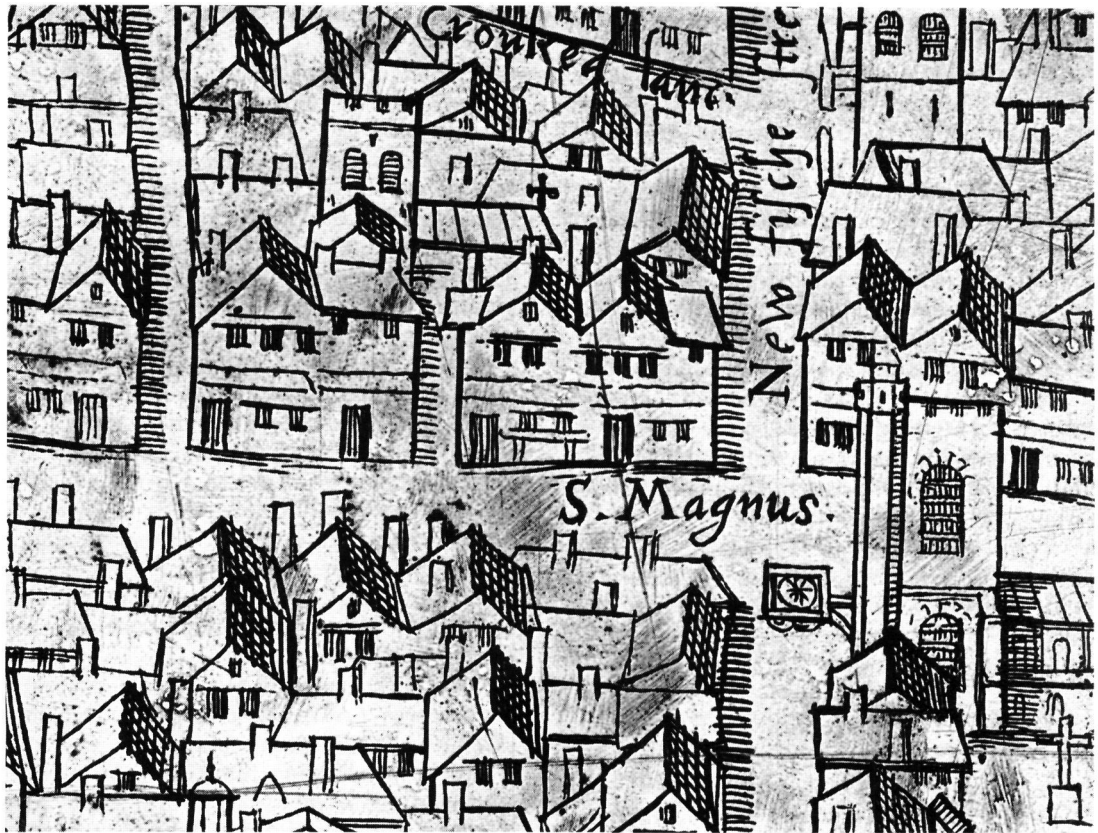
FIG 4 The Copperplate Map of c. 1557 (detail). In the building immediately above 'S. Magnus', the penthouse roof and stallboard on legs denote a shop. (Museum of London).
