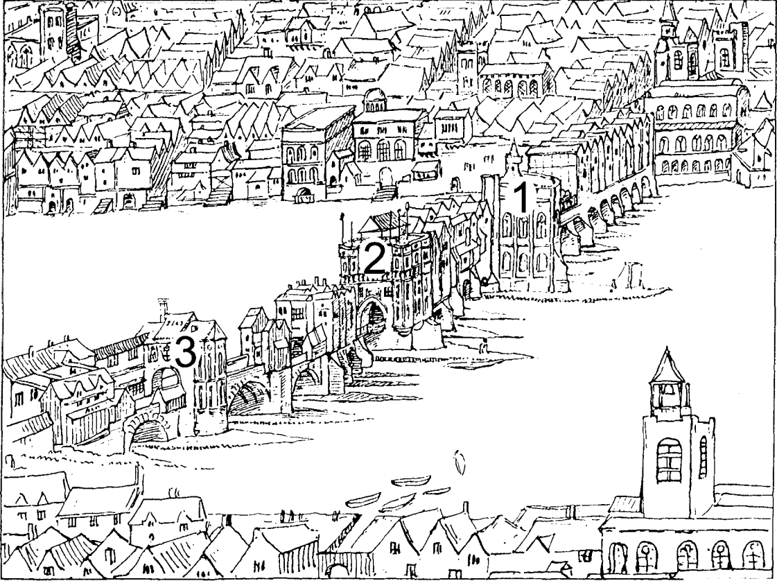
Fig 6. Medieval London Bridge looking north-west showing the chapel of St Thomas (1), the Drawbridge Tower (2) and the Stonegate (3). This view is based on a portion of Wynegarde's panorama of c.1544
