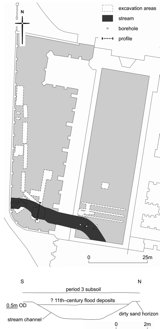
Fig 4. Cromwell Green: plan (1:1000) and reconstructed profile (1:150) of the excavated Period 1 channel, with a projection of its course beneath Westminster Hall, based on window sample and borehole evidence
