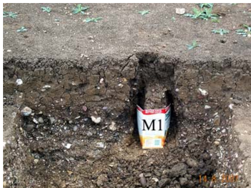
Plate 19. Trial-pit C, Box-section D (south face). Monolith sample M1 through palaeosol and base of alluvium (see Appendix 6)
