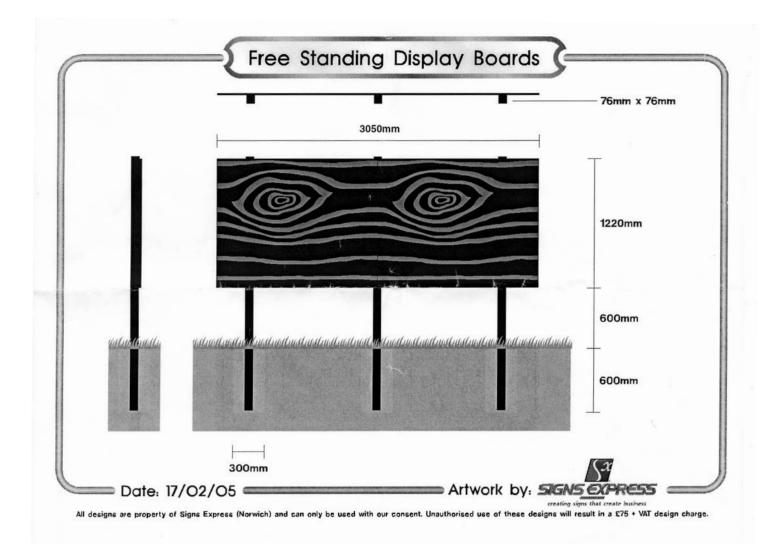
Figure 3. Design of display board
