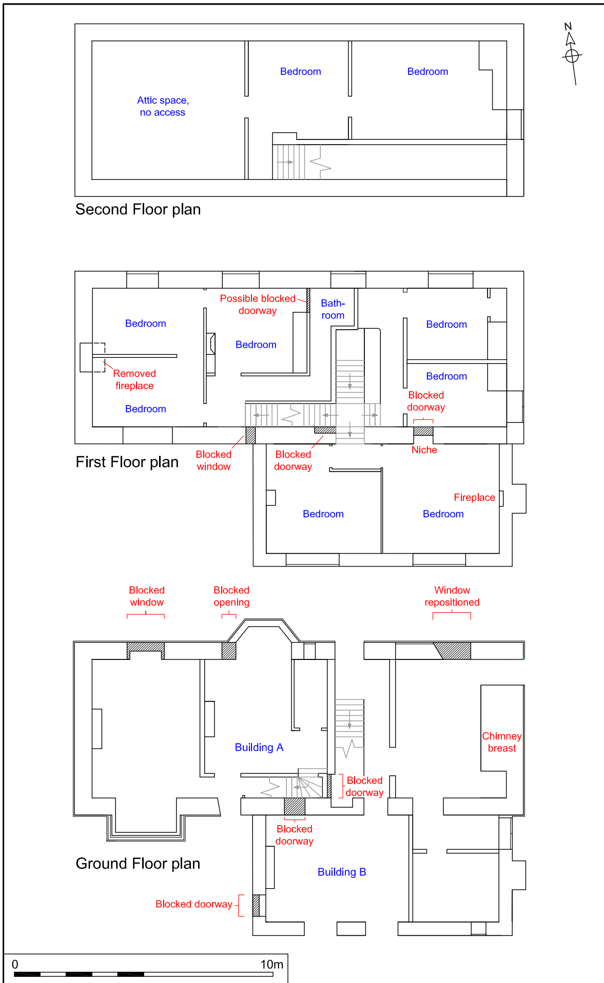
Figure 3. Plan of Buildings A and B. Scale 1:150
