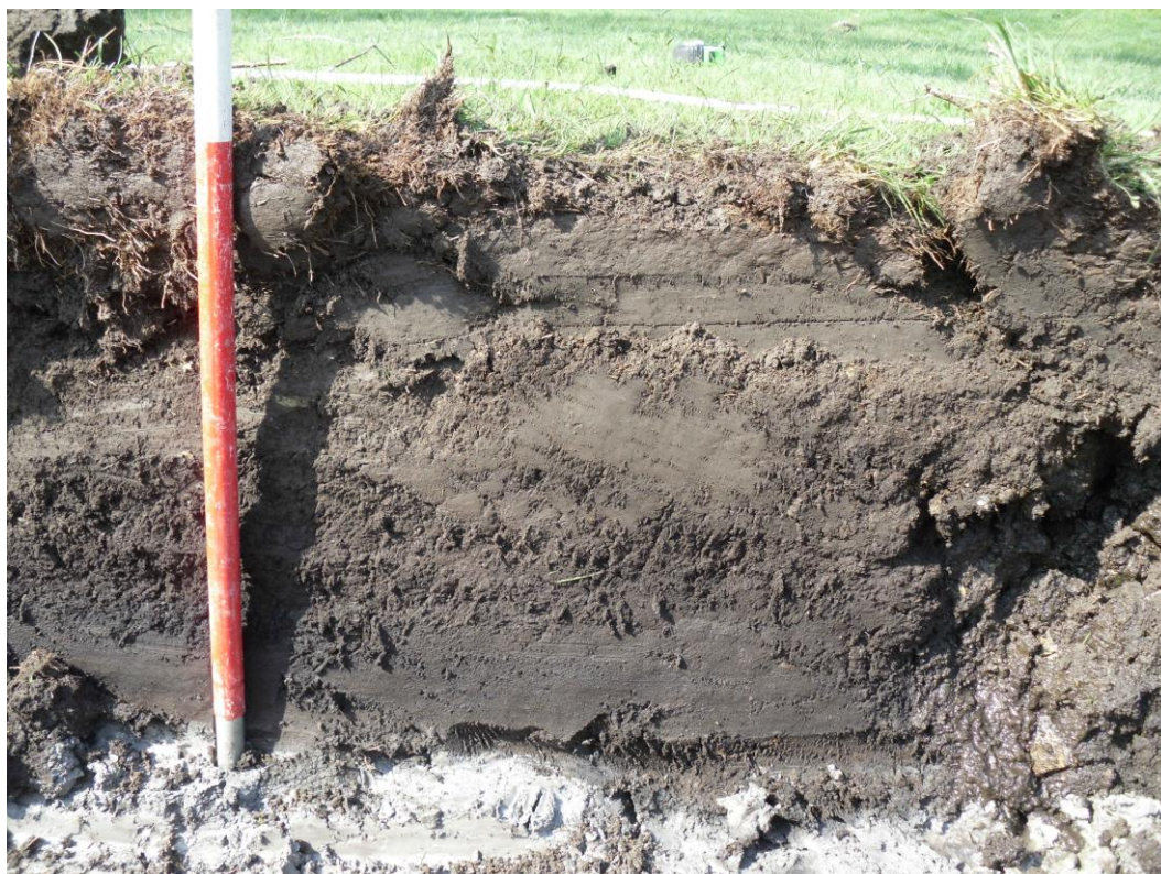
PLATE 1 Typical section showing thin topsoil/turf, over peat over glacial clays
