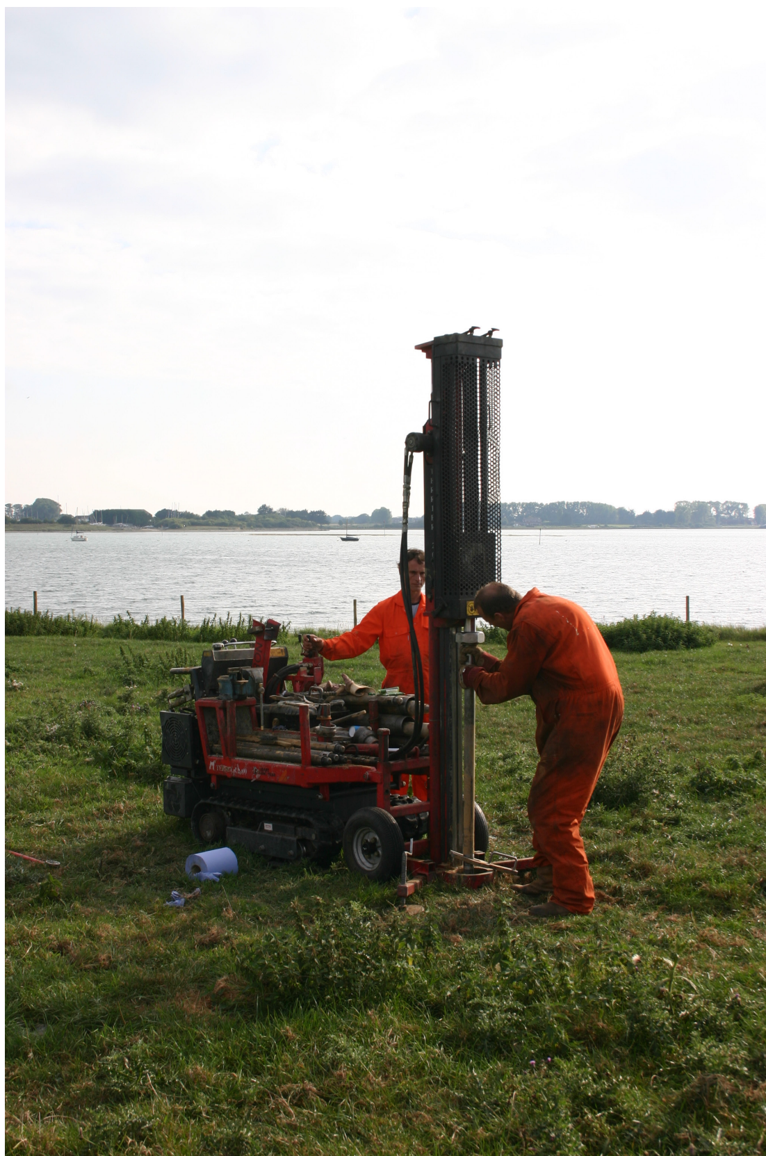
Plate 1. Terrier drill rig of type used at Pulborough.
