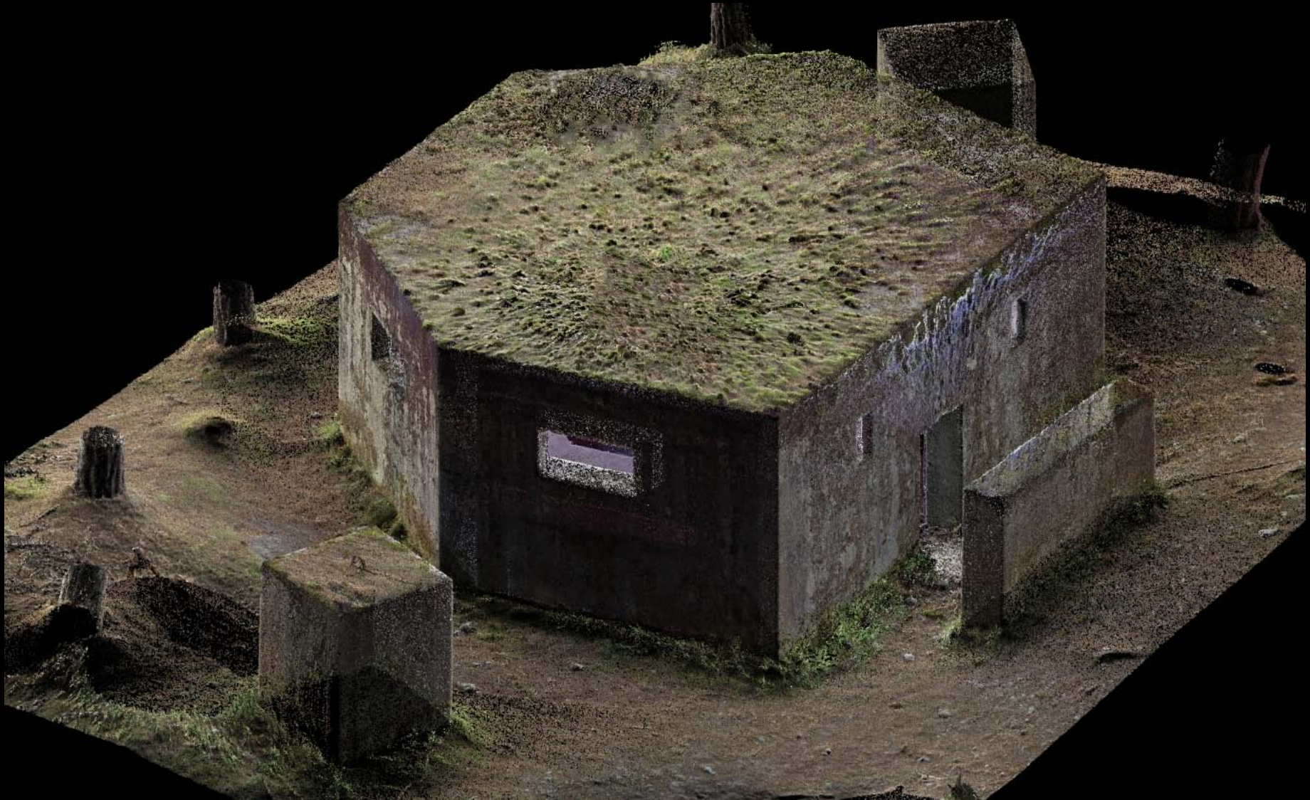
Figure 15: Orthoimage of the laser scan pointcloud showing the south side of the pillbox with its entrance and anti-blast wall, with real colour and edge lighting, from above S
