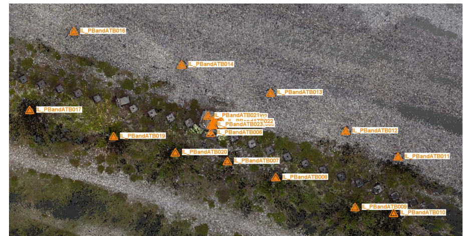
Key plan showing locations of scanner stations during survey of Lossie Forest Rectangular Pillbox and Anti-Tank Blocks
