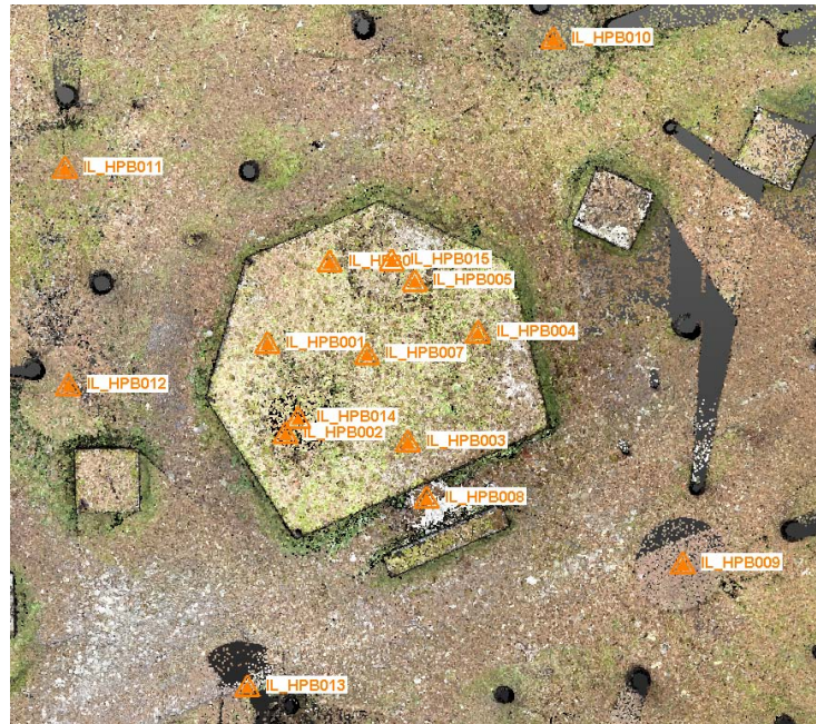
Key plan showing locations of scanner stations during survey of Lossie Forest Hexagonal Pillbox
