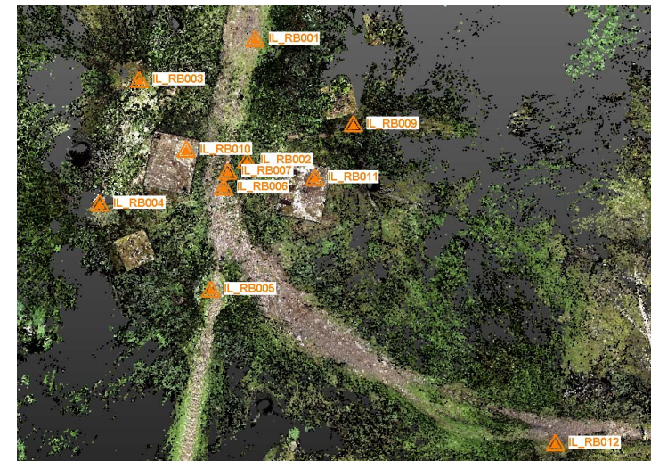
Key plan showing locations of scanner stations during survey of Lossie Forest Road Block
