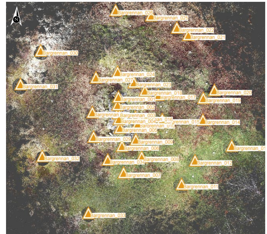
Key plan showing locations of scanner stations during survey of Bargrennan cairn
