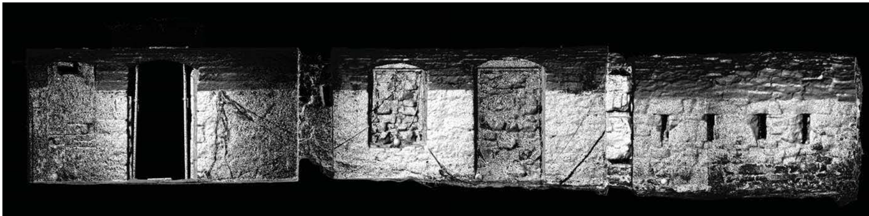
Ortho-image of the north-west vault Interior elevation, using intensity values and lighting
