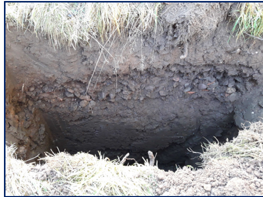
Plate 2: Field drain in geological test hole
