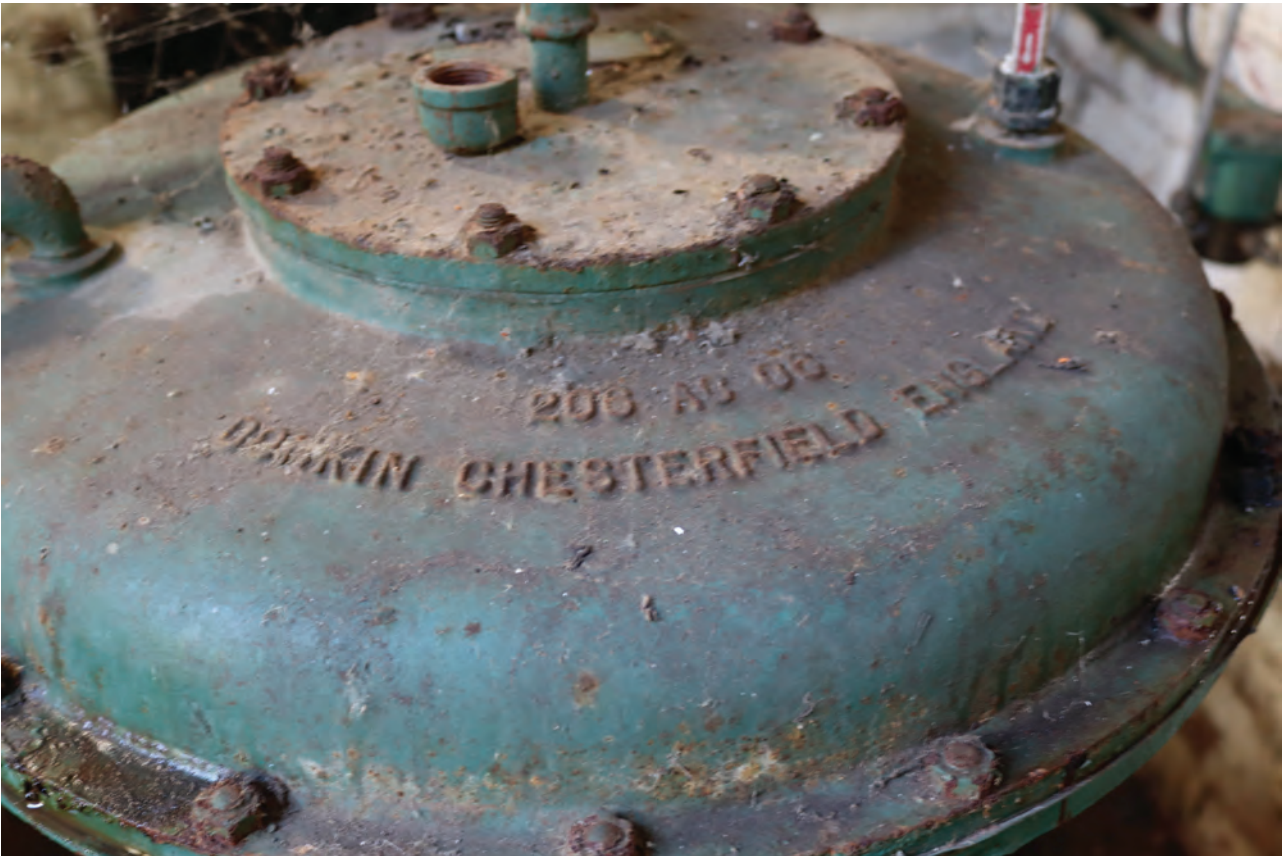
Plate 143: Structure N, detail view of 'DONKIN' maker's mark on the volumetric governor, from the WNW
