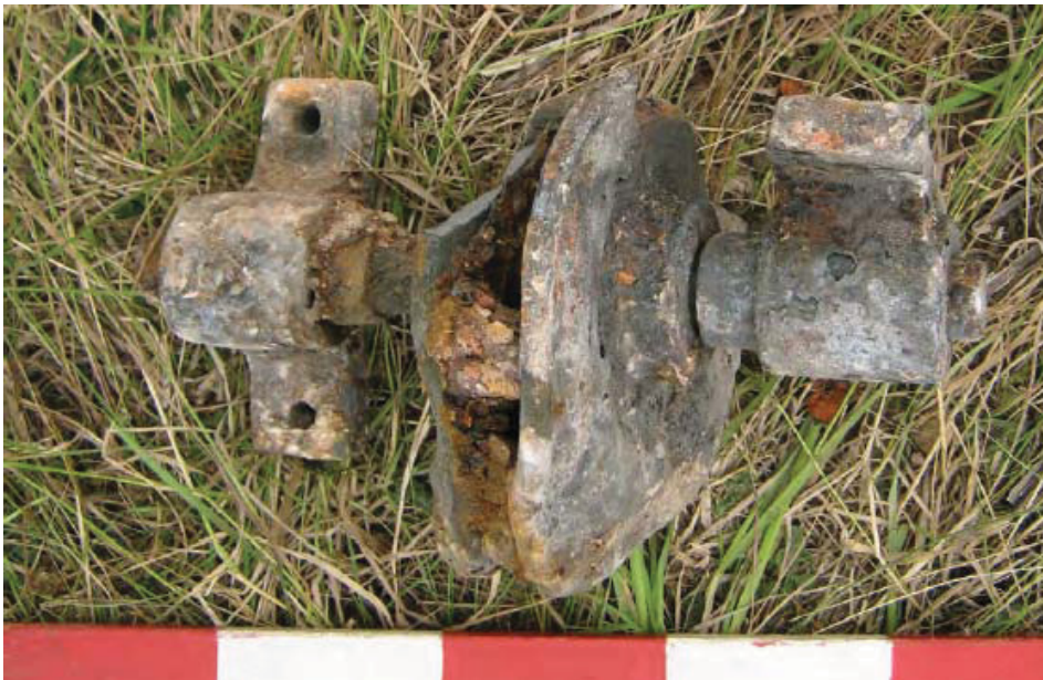
Figure 6. Bearing, shaft and pulley assembly. Note fixing holes in bearing housing.
