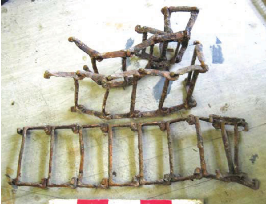
Figure 13 Sections of the ladder link conveyor.
