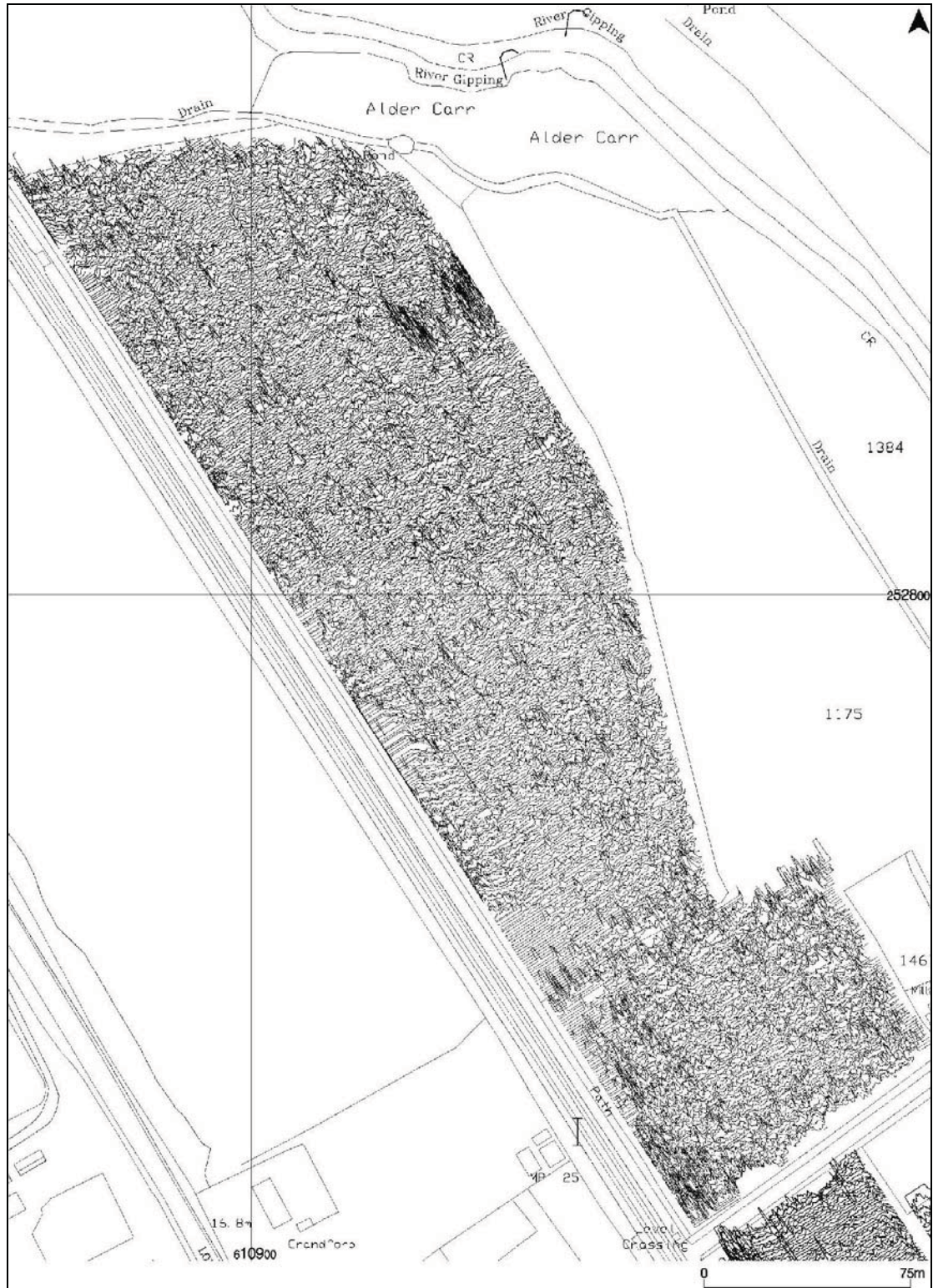
Figure 7. XY trace plot of raw gradiometer data; Block 1
