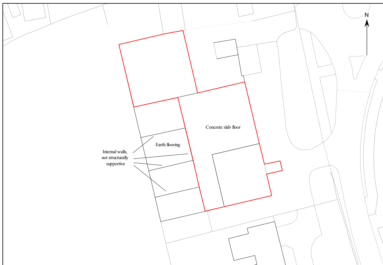
Figure 4. Internal structure of barn, showing concrete slab floor (outlined in red)
