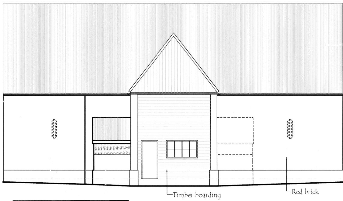
Figure 6 Western external elevation showing original ventilation loops and hipped porch (now blocked by 20 th century weatherboarded studwork). The northern lean-to shed to the left is also original but its walls were later raised (shaded) and its southern counterpart (indicated by broken lines) has been demolished. Adapted from a drawing provided by Clarke & Simpson. Scale in metres.
