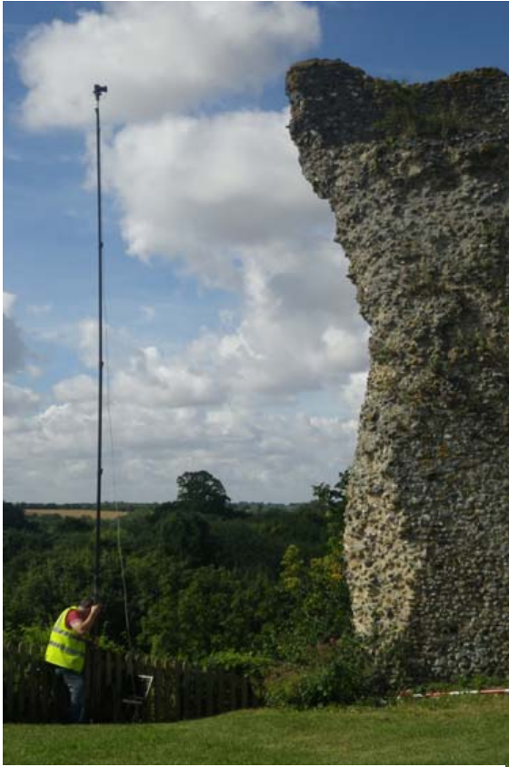
Plate 3. Derek Ashman from Higher View Ltd. photographing the keep using a camera mounted on a telescopic pole
