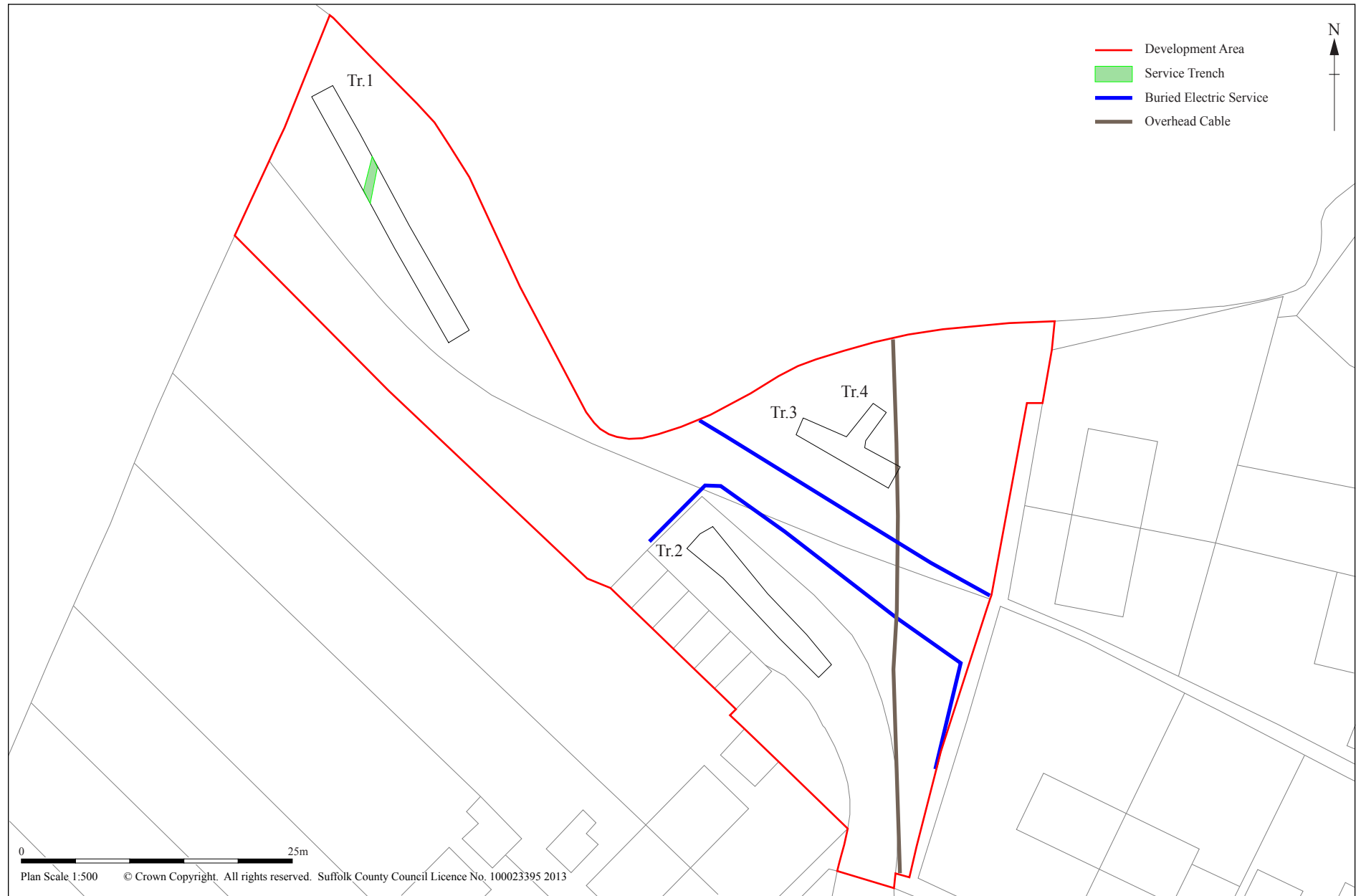
Figure 2. Site plan, showing trenches and services
