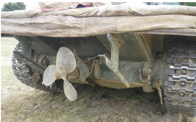
Fig 3 Close up of rear propeller on a Valentine DD – power is taken direct of the gear box
