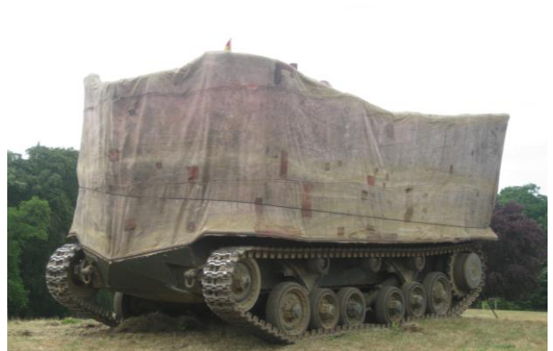
Fig 2 Valentine IX DD with Screens inflated. This tank is the only surviving example of a Duplex Drive Valentine
