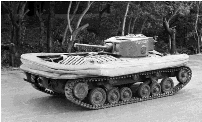
Fig 1 Valentine DD at Gosport 14 th January 1944 with screens down. Note the turret is 180 degrees to the rear, so as not to foul the screens
