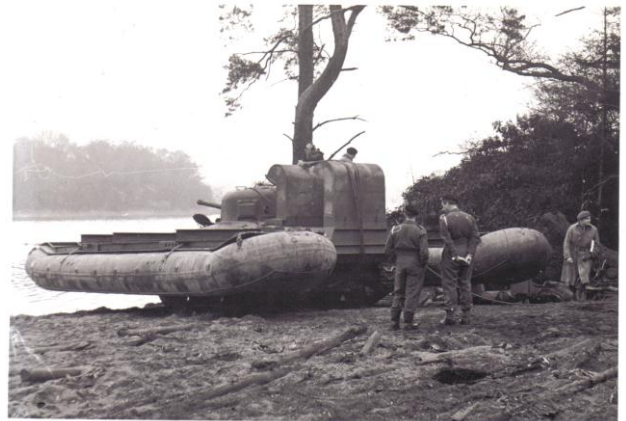
Fig 35 M12 Floatation Device – Trails at Fritton 1946 [SEPA 6681/04/09]
