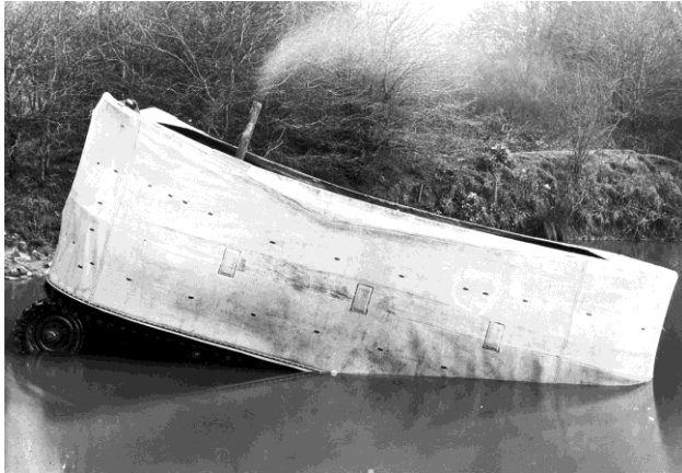
Fig 32 Valentine DD being tested for waterproofness in Fritton Immersion Pool [Bovington 2191-E1 ]
