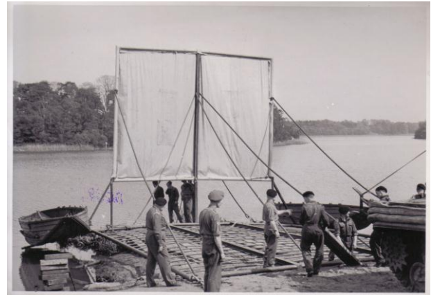
Fig 24 "Ginandit Mk II" was a device used to push in front of the tank whilst swimming and deployed over soft mud. SEP 6681/04/09
