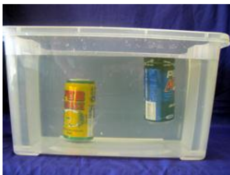
Fig 4 Demonstration showing that the can containing more sugar is denser than diet or zero sugar drinks. In this case, the drink on the left contained 46g of sugar, compared to 2g in the right hand can.
