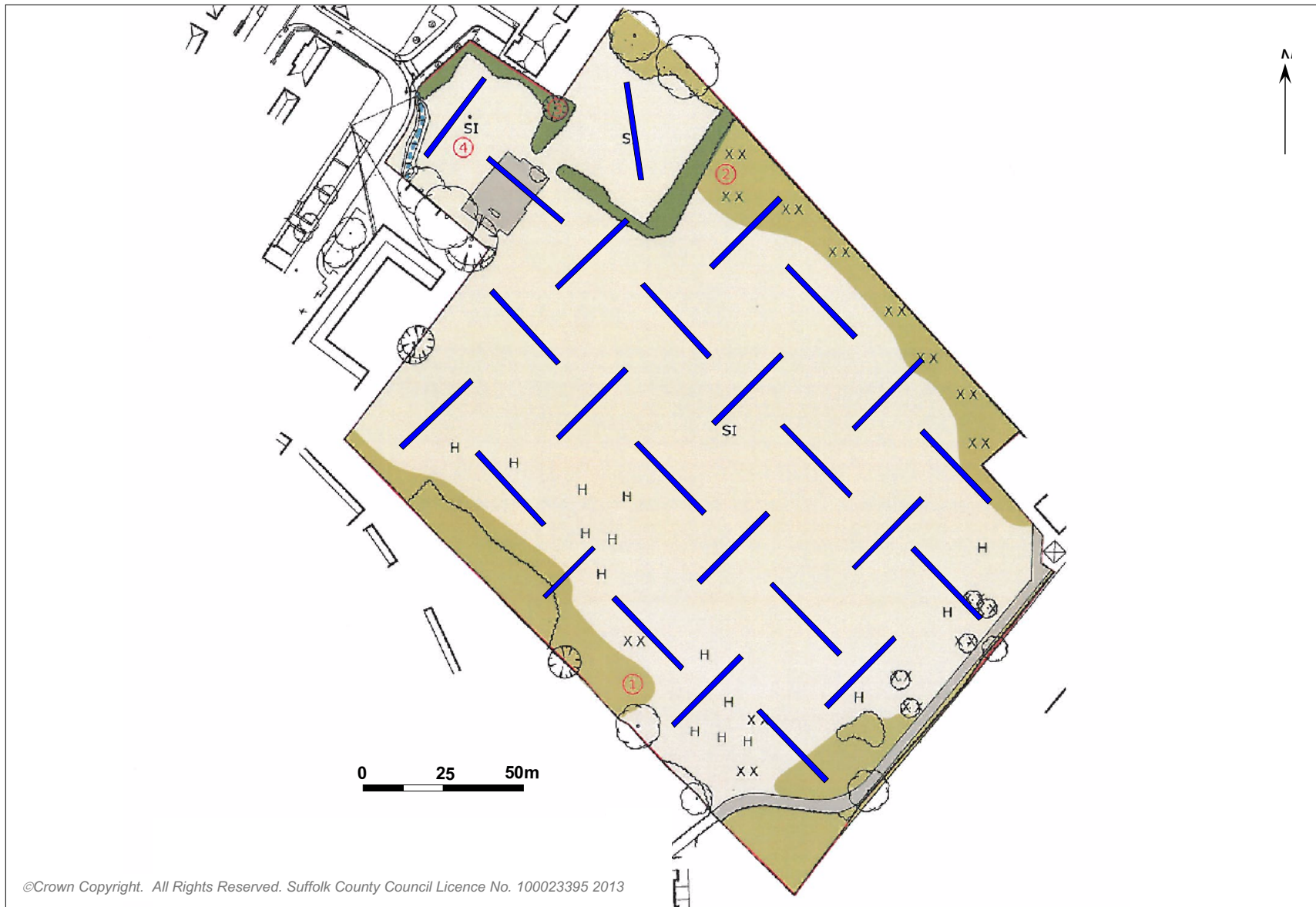
Figure 2. Site detail and proposed trench locations (“H” legend denotes heather – to be undisturbed by trenches or associated spoil)
