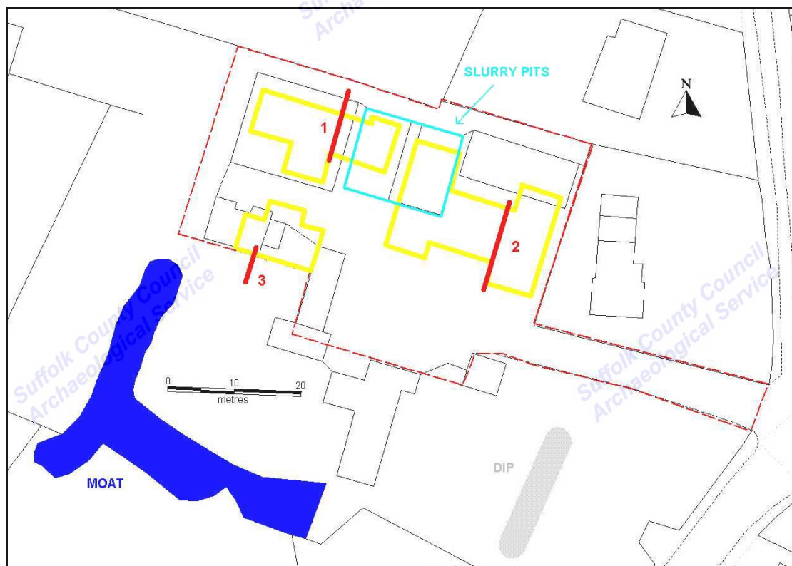
Figure 3: Trench plan showing the total site area (dashed red line), the brick-lined slurry pits (light blue), the existing section of the moat (dark blue) and the proposed new buildings (yellow).
