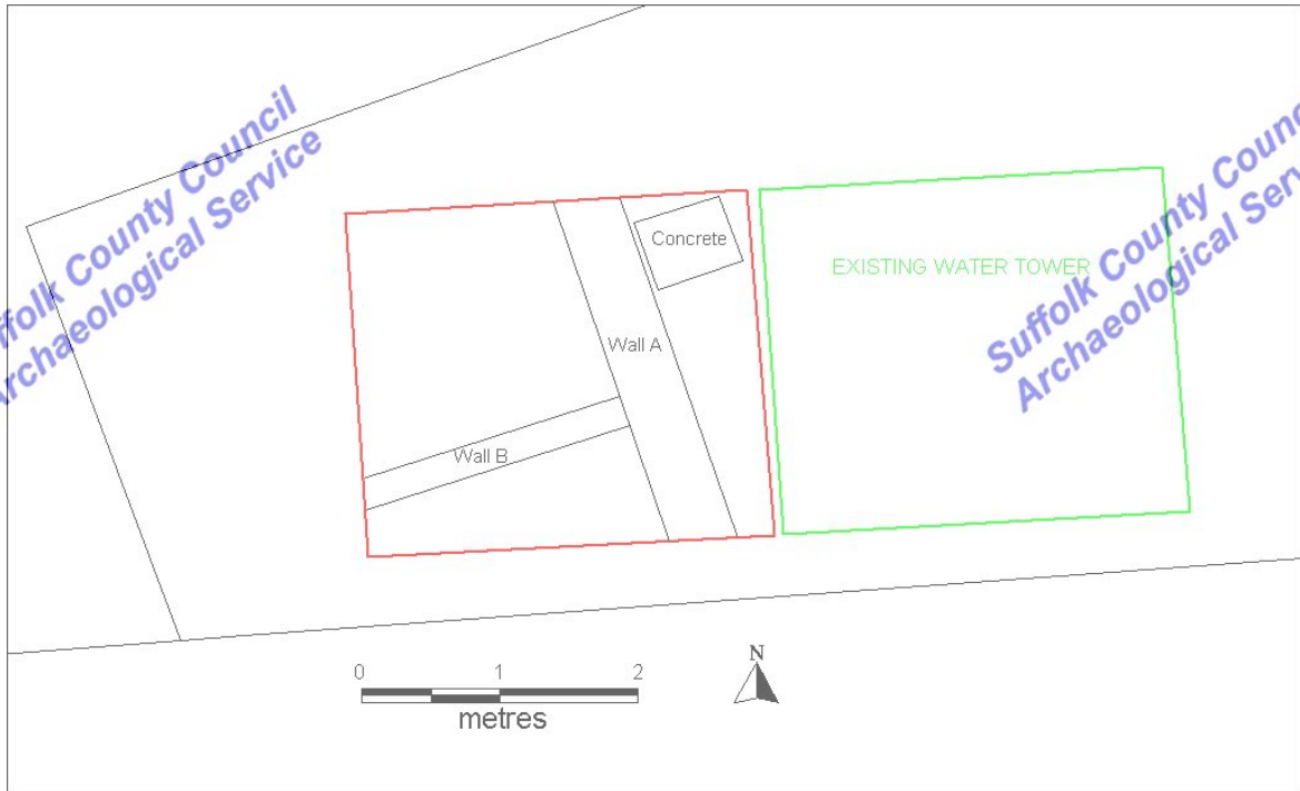
Figure 2. Plan showing the trench outline (red) the site of an existing water tower (green) and the location of the brick foundations
