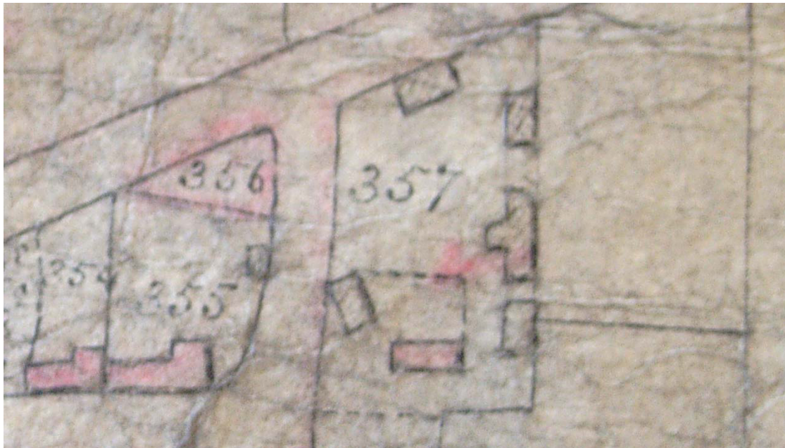
Figure 2a. Detail of 1839 tithe map above, showing the house in pink to the south and the detached 'dairy' wing at an angle to the east. The map is not fully accurate, as indicated by the exaggerated degree of this angle, but the barn is clearly shown with a central porch or lean-to against its eastern elevation, and the granary is a detached structure to the south. The two buildings at the northern end of the site no longer survive.
