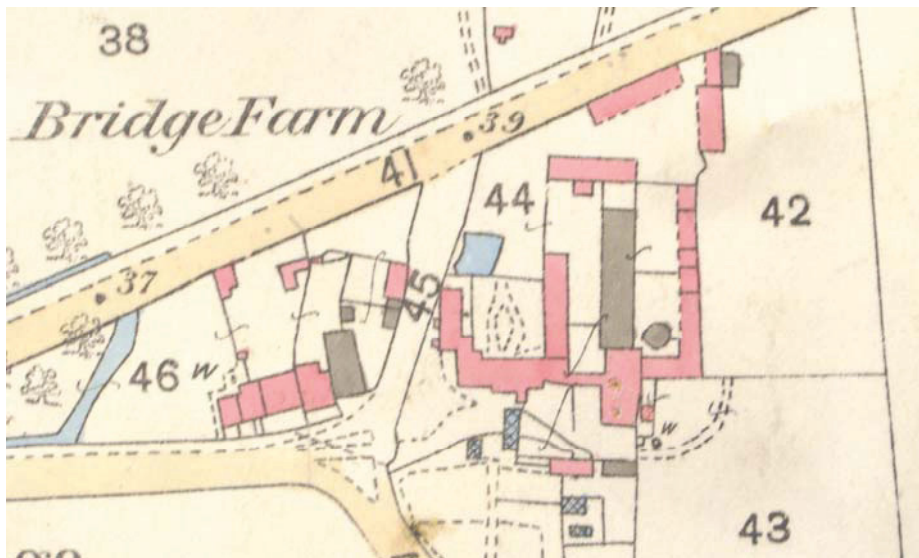
Figure 3a Detail of the first edition 25 inch Ordnance Survey of 1883 above, showing the much enlarged mid-19 th century farm complex. Red is used to depict domestic and masonry structures as opposed to utilitarian and timber buildings, and reflects the brick external walls of the southern granary. The cattle yards and sheds to the east of the timber-framed barn no longer survive.
