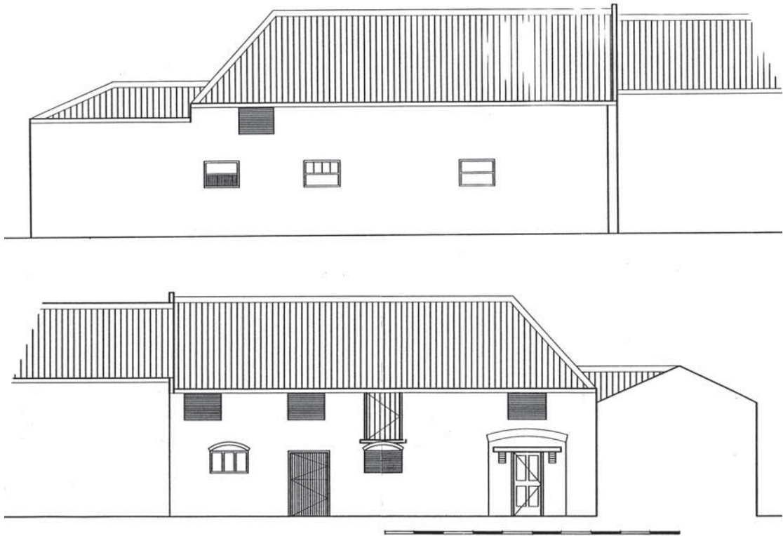
Figure 5 External northern (top) and southern elevations of the 19 th century stable and former coach house (scale in metres, omitting brick dressing). Drawn by Brown & Co. of Norwich. The arch of the coach house door is shown to the right. The left door was moved from the left-hand window to the centre of the new range in the mid-19 th century when the early-19 th century stable was extended.
