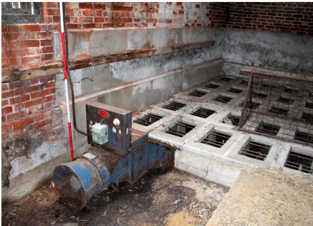
Illus. 10. Detail from south of mid-20th century grain sack dryer in floor of barn (1).
