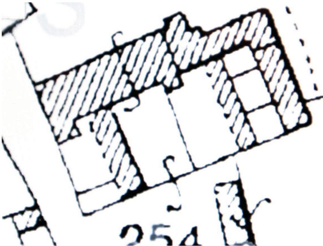
Figure 5. The farm complex on the second edition 25 inch Ordnance Survey of 1904 showing a new, central shelter-shed that no longer survives to the south of the barn. The western elevation of the eastern shelter-shed (3) is not shown as open-sided having perhaps been enclosed to form loose-boxes.
