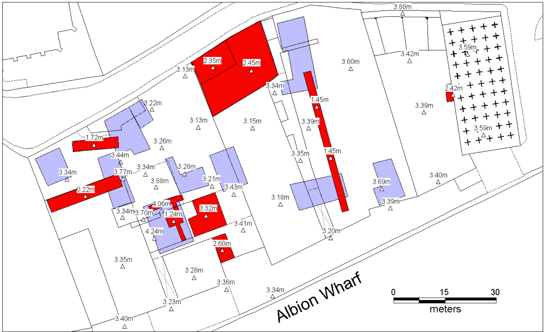
Figure 10. Principal floor and slab levels
