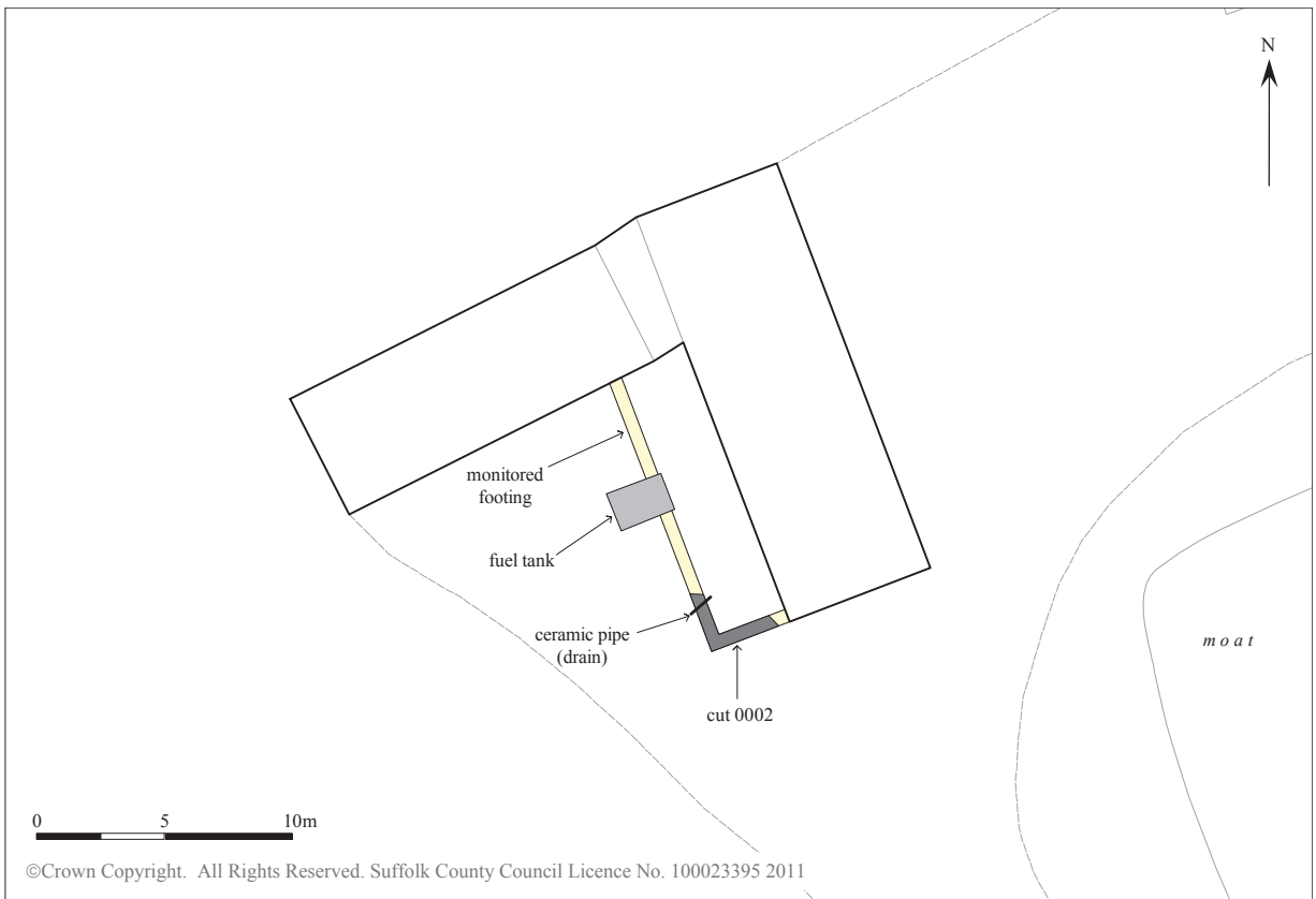
Figure 2. the monitored foundation trench
