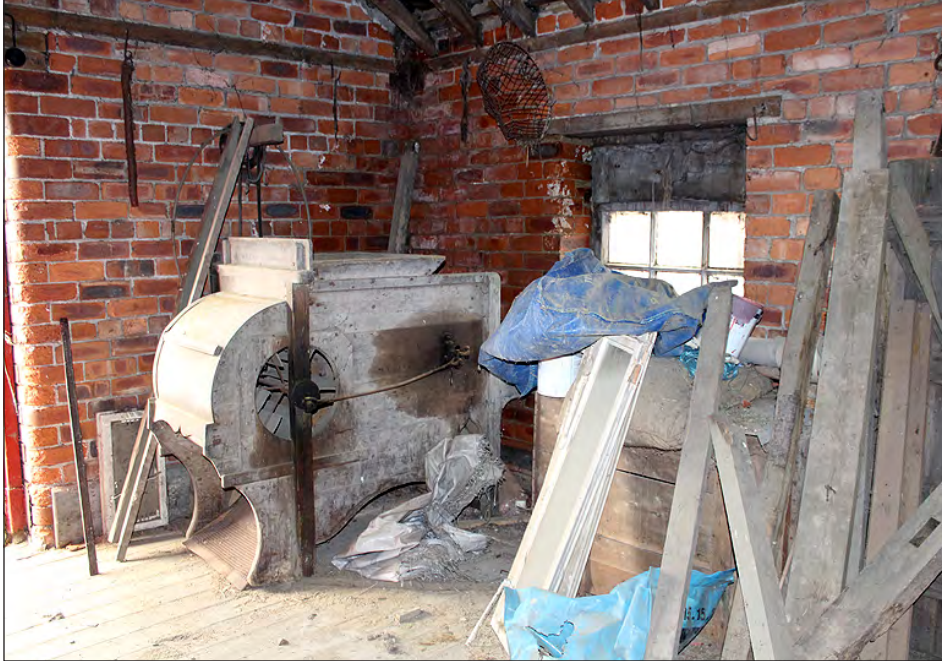
Plate 35. Building 3, interior. Winnowing machine. View looking northwest
