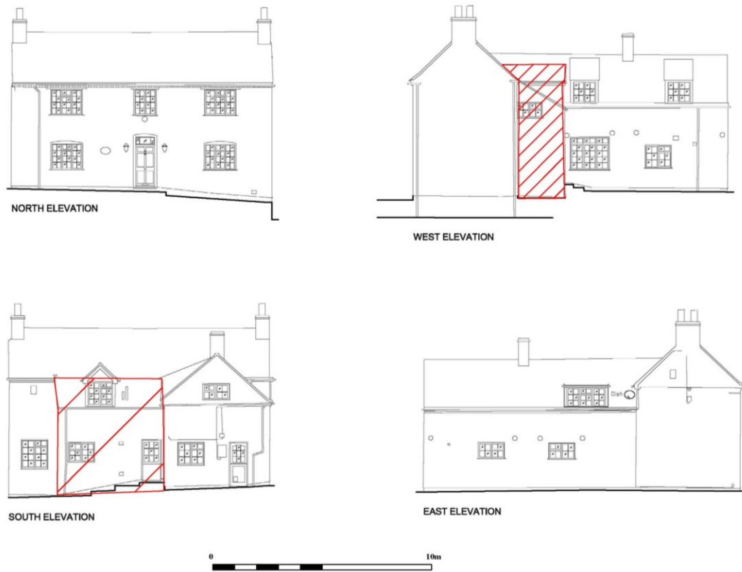
Figure 4 Existing elevations Demolished extension highlighted in red. Source: HSSP Architects/Mr and Mrs Cheetham
