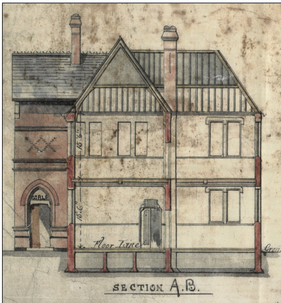
Figure 7. Extract from LBR Plan 1873/2703, showing architect's original cross-section drawing of Oxford Street School. Not shown to scale.
