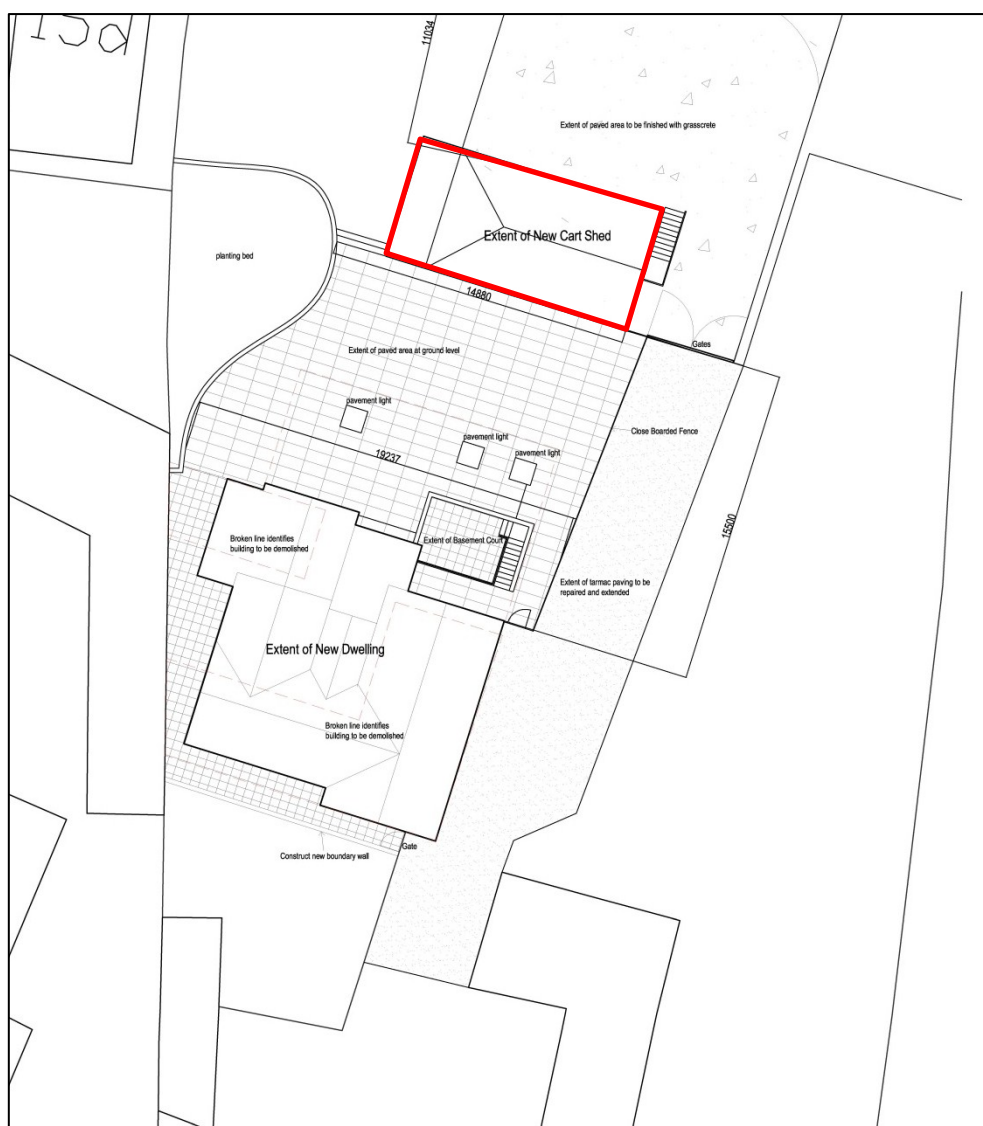
Figure 2. Location of proposed new cart shed (outlined in red) to the rear of Cresswell Spring Farm (supplied by Mr. Pilkington, not to scale).
