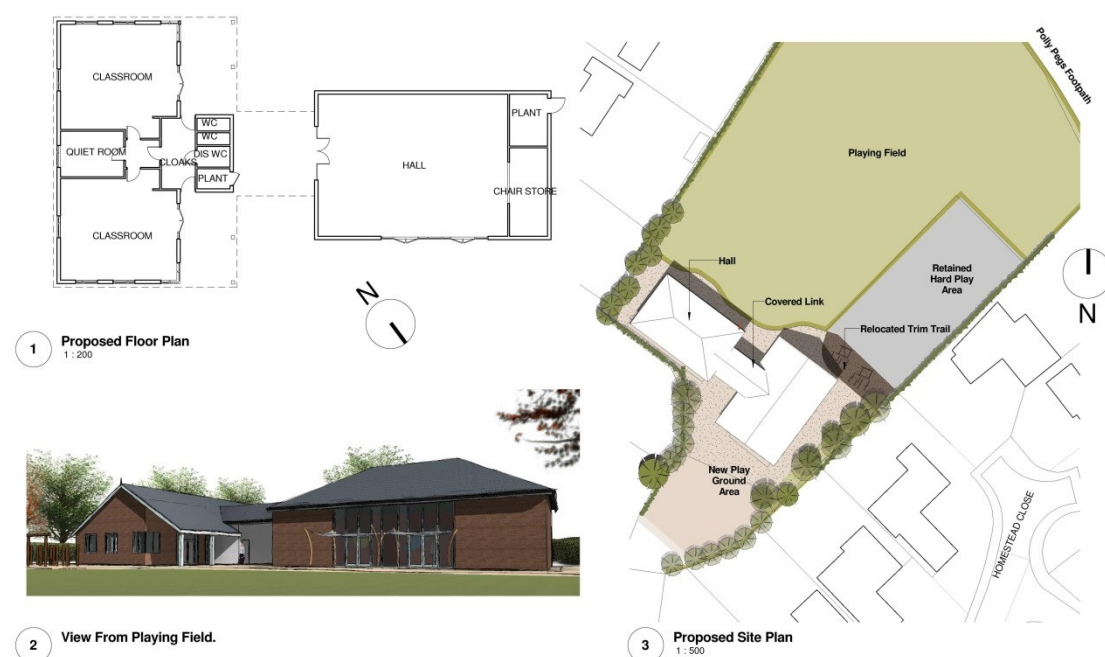
L1501 New Classrooms and Assembly Hall SK01 Sketch Plan and Perspective View
