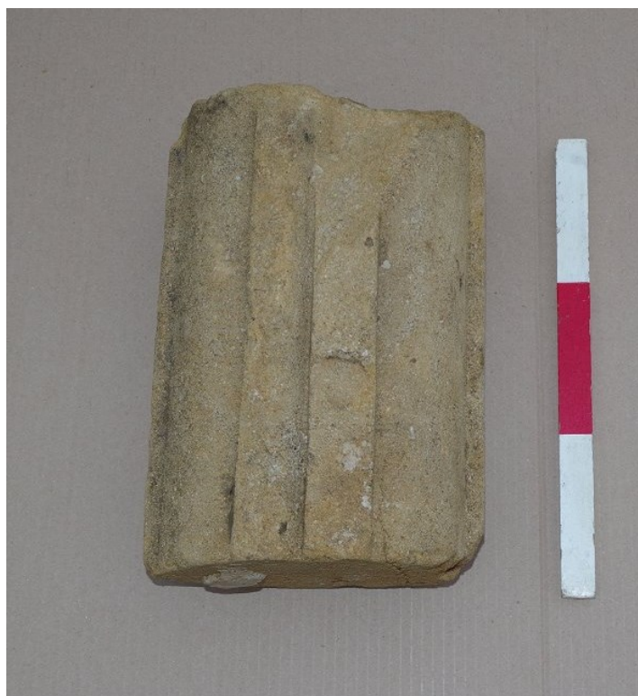
Figure 23. Window mullion A, ovolo-profile. Scale 300mm.
