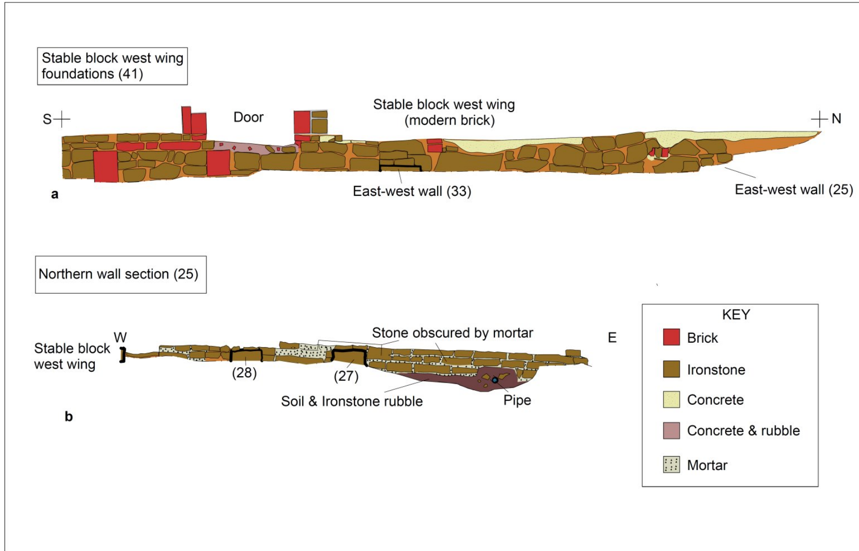
Figure 10: Sections of foundations and wall recorded in 2005
