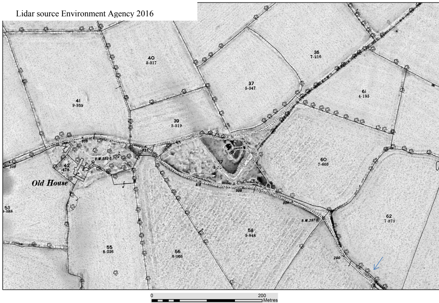
Figure 25: RVT positive openness analysis of the 1m DTM LiDAR data, with Hartley's earthwork survey, and 1 st edition Ordnance survey County Series mapping 1:2500, 1886. Rising stream is arrowed in south-west. Possible ridge and furrow visible to immediate north-west, south and east of the fishpond.
