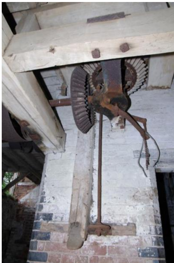
Figure 29 Building B ground floor south room millstone drive gears Looking north. Note wooden chute for milled material
