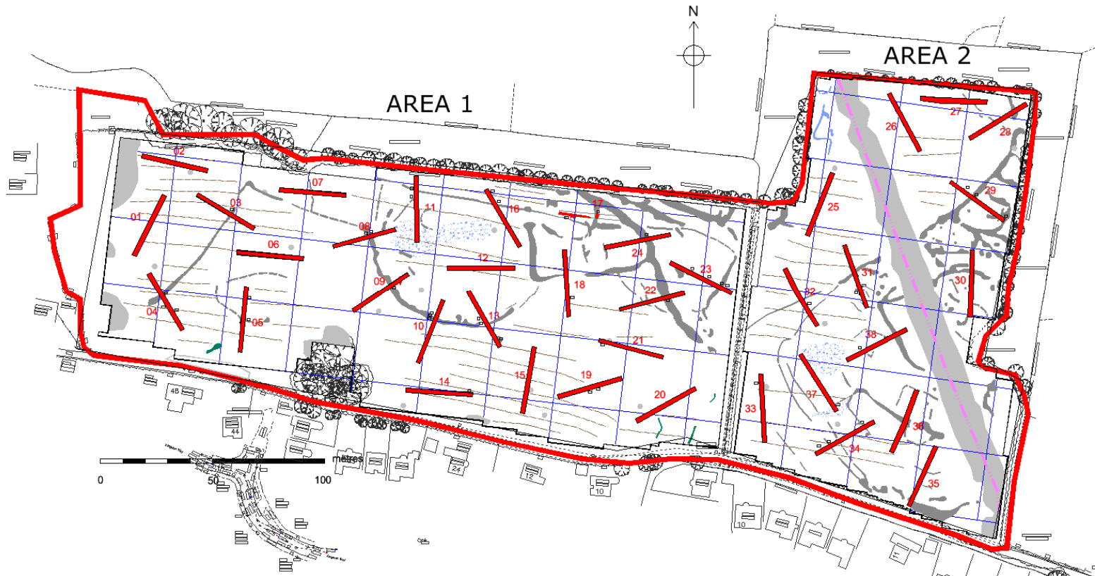
Figure 4: Trench plan overlain on the geophysical survey. The pale grey diagonal line in Area 2 indicates a 10m stand-off for the service trench.
