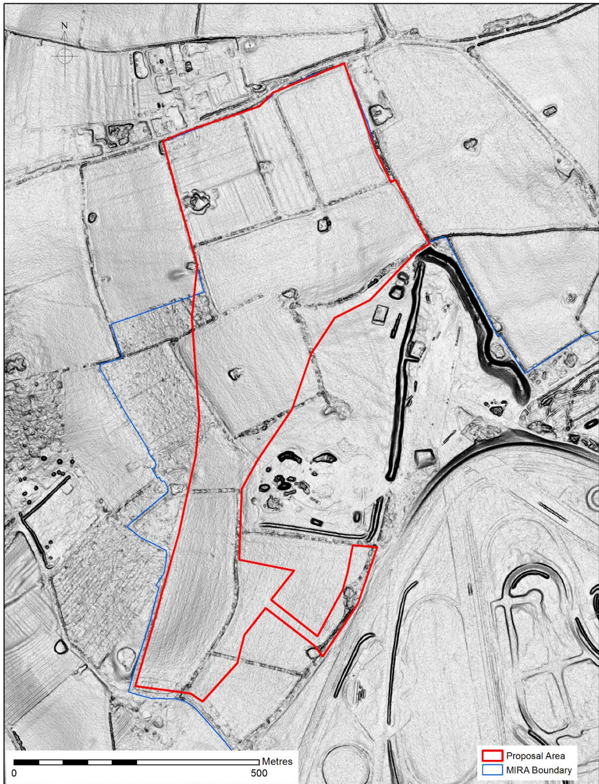
Figure 8: Results of LiDAR assessment showing Slope Analysis plot of 1m DTM data.
